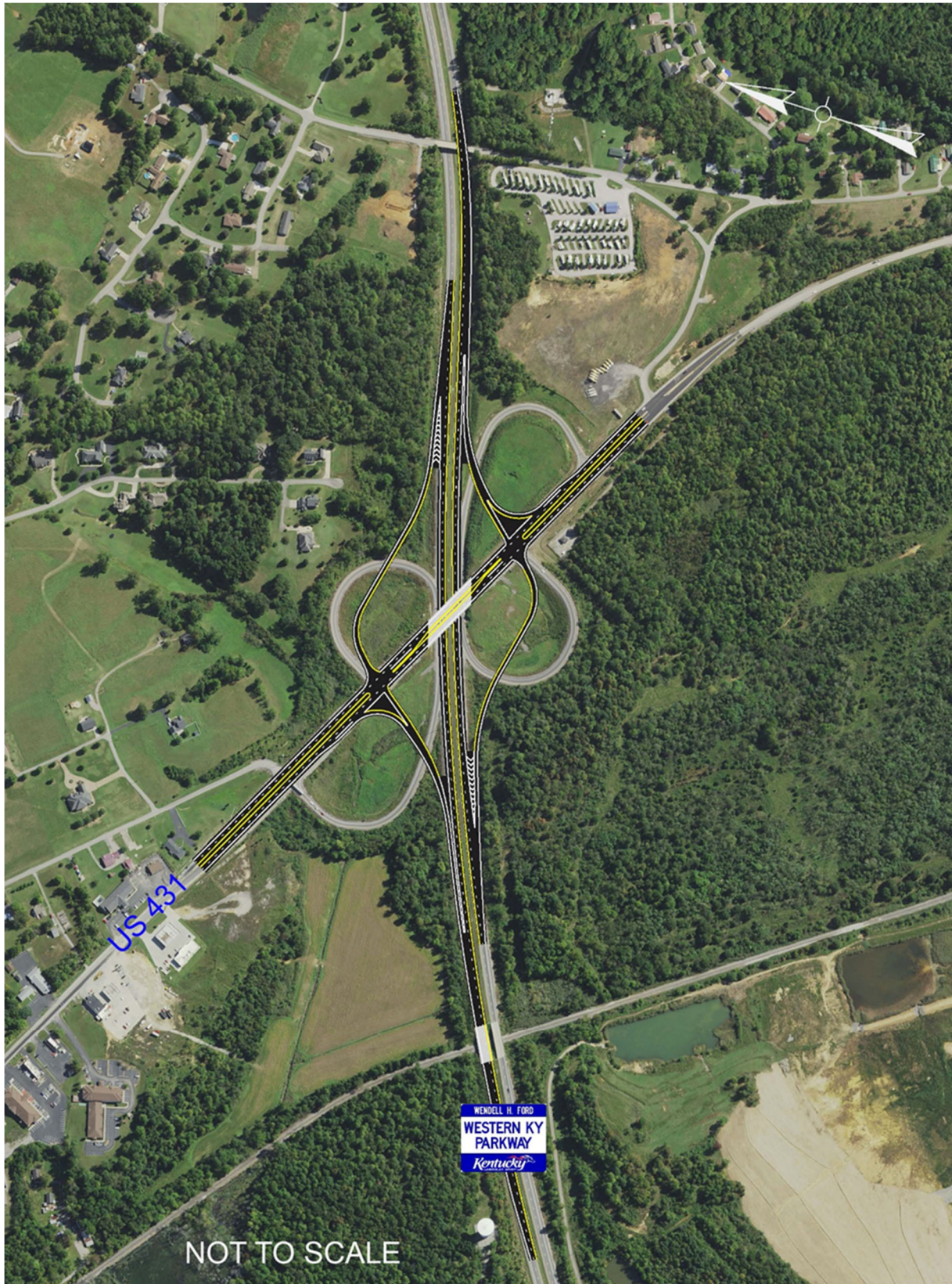
Figure ES-3. US 431 (Exit 58) Interchange Reconfiguration
